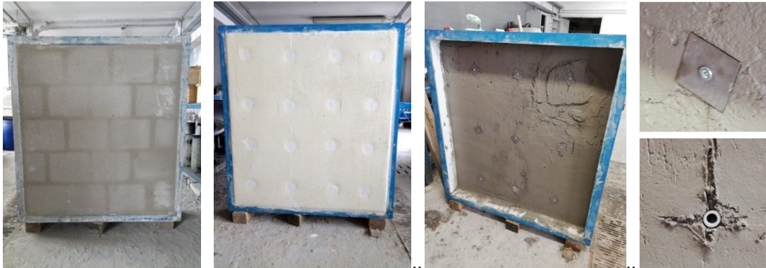
Figure 1. From left to right: the test wall proton side (internal) and insulating side (external), the connections for fixing the SFRM coating.
