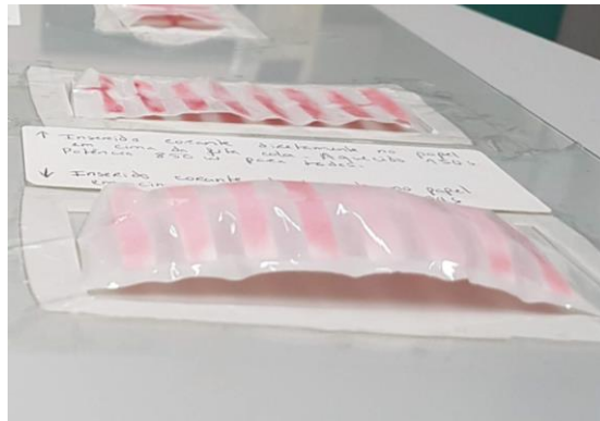
Figure 3.9 - Actuator tested during 1 minute in the microwave oven at 800 W.
