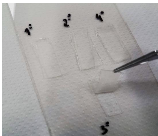
Figure 3.7 – Experiment of the adhesion between PDMS and Ecoflex 30 after UV treatment: 1) both PDMS and Ecoflex 30 with UV; 2) only Ecoflex 30 with UV; 3) only PDMS with UV; 4) PDMS and Ecoflex 30 with UV and PMMA between them without treatment.
