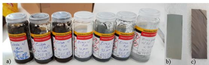
Figure 3.13 – a) The solution of the metallic nanoparticles: copper 40 nm; zinc 10 \mu\text{m} and zinc <150 \mu\text{m} ; b) paper with gold nanoparticles and c) silver nanowires with fibrillated cellulose fibers.
