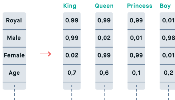
Figure 2.3: We can easily see what each dimension might mean in these embeddings and the reason why these are useful in relative comparison scenarios [22].
