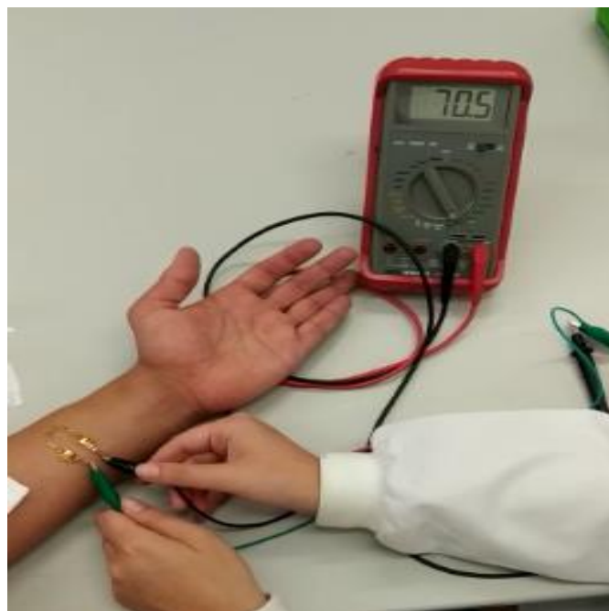
Figure 6.9 - Measurements of resistance, while the sensor is attached on-skin.
