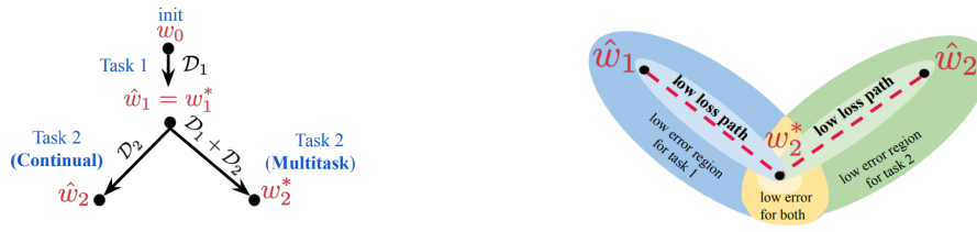
(A) First, \hat{w}_1 is learned on task 1. Then, we either reach \hat{w}_2 by fine-tuning second task or w_2^* by training jointly on both tasks. (B) Linear connectivity between w_2^* and \hat{w}_1 and between w_2^* and \hat{w}_2
