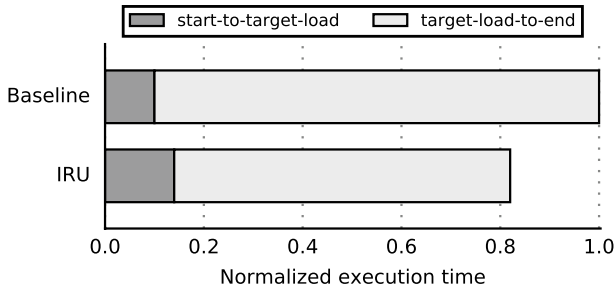
Fig. 3 Warp average normalized execution with and without IRU. The dark bar indicates execution time until the target load is serviced, and the light bar from service to finalization. Processing a load instruction with the IRU is slower as it has to reorder data elements to identify indices that target the same cache line. However, once the indices are sent to the SMs, the remaining execution is faster as subsequent memory accesses used the IRU-prepared indices that result in higher memory coalescing
