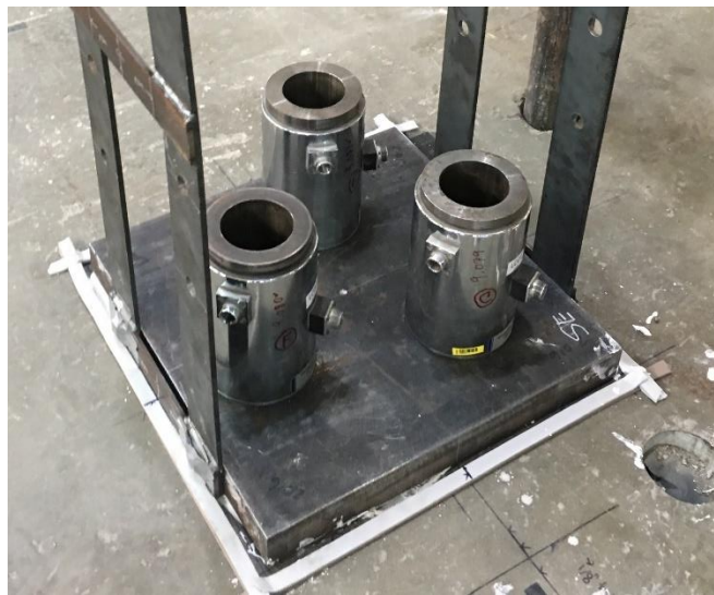
Figure 4.28 Load cells in the support fixtures
