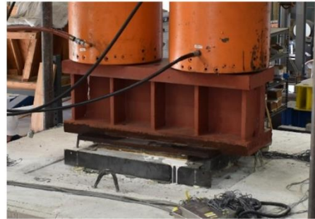
(b) Spreader beam after setup
