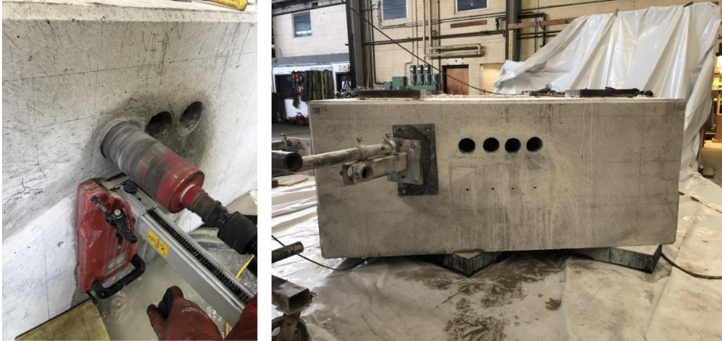
Figure 6.7 Coring work (left) and position of coring on the north face of the specimen (right)
