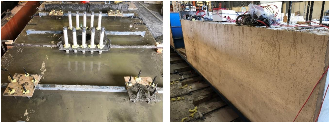
Figure 6.6 Bleeding occurred in batch #3 (left) and surface of the specimen after curing (right)
