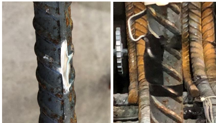
Figure 5.11 Polished longitudinal rib (left) and minimized protection area (right)
