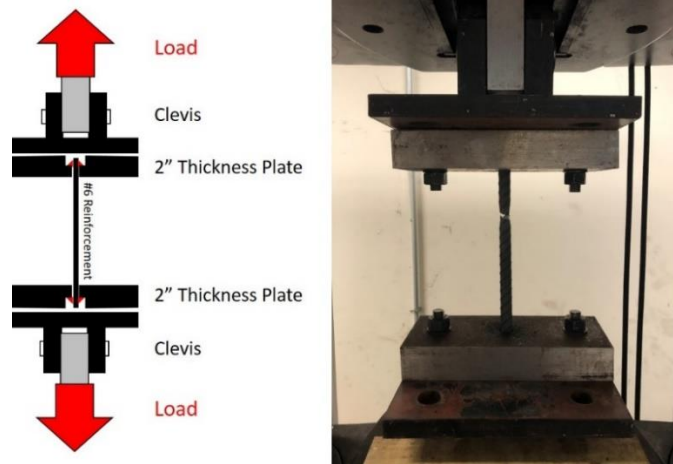
Figure 6.10 Mock-up test plan (left) and fracture of reinforcement after mock-up test (right)
