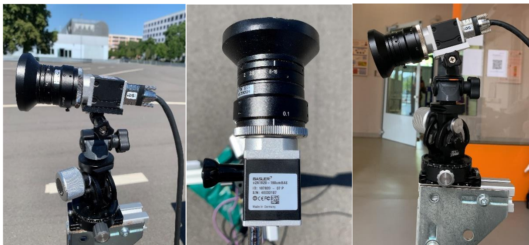
Fig. 31 – Camera for radar image support
