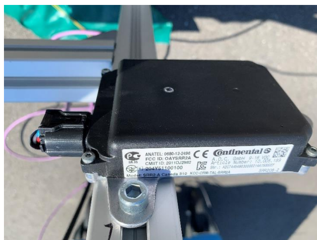
Fig. 37 – SRR 20X 24 GHz short-range radar sensor manufactured by A.D.C. GmbH
