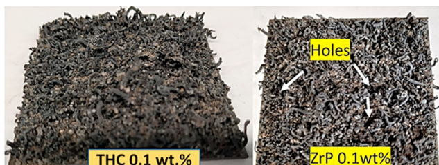
Fig. 2 – Physical appearance of coating char of THC 0.1wt% and ZrP 0.1wt%.
