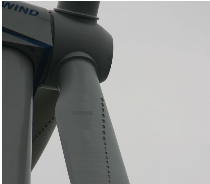
Figure 21: VG array mounted onto an actual wind turbine blade. [56]
