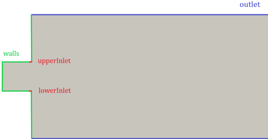
Figure 23 Boundary conditions of the main case geometry, Source: Own
