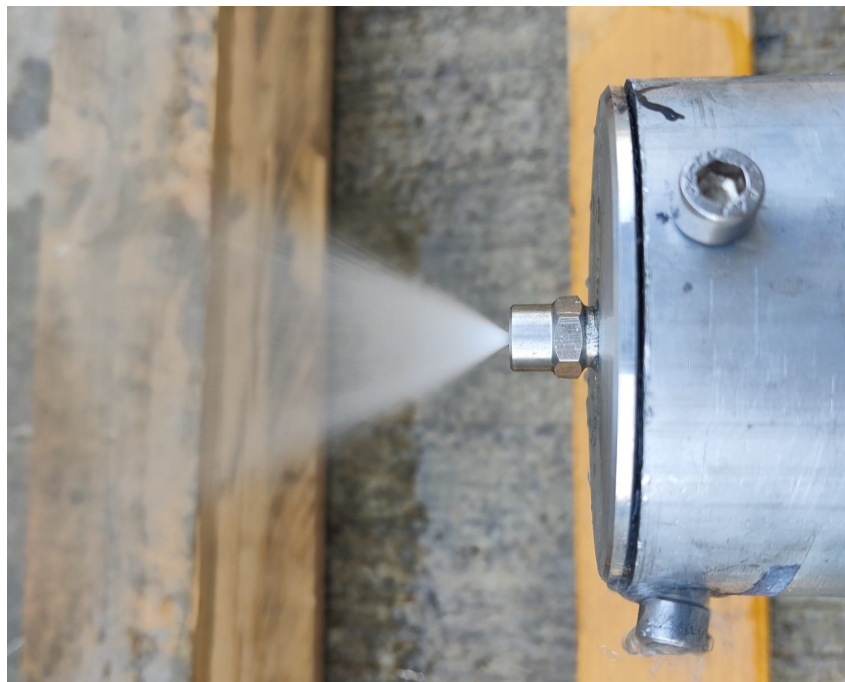
Figure 65 Solid cone nozzle spray pattern, Source: Own
