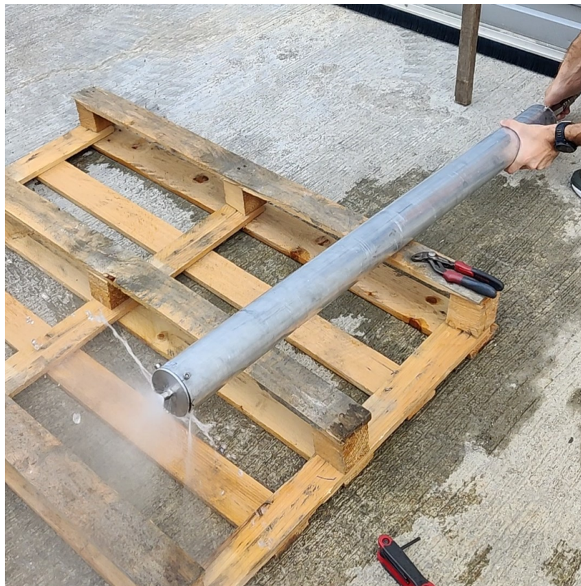
Figure 67 Prototype cover sealing malfunction, Source: Own
