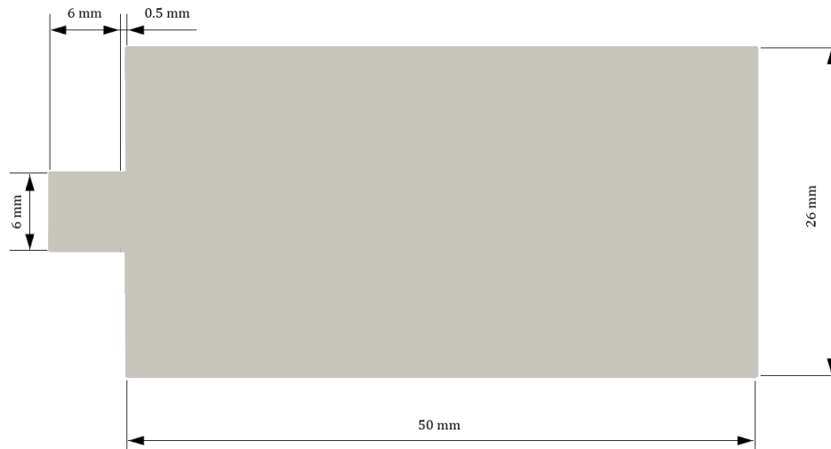
Figure 19 Geometry of the doublet injector simulation, Source: Own
