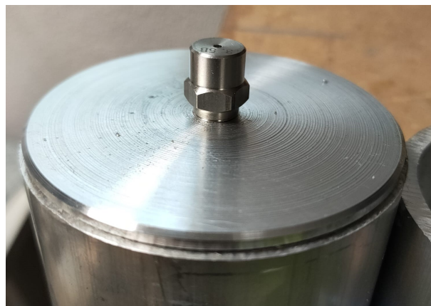
(c) Stream nozzle installed
