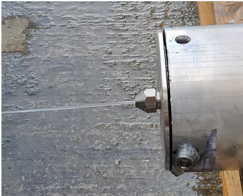
Figure 68 Solid jet nozzle spray pattern, Source: Own
