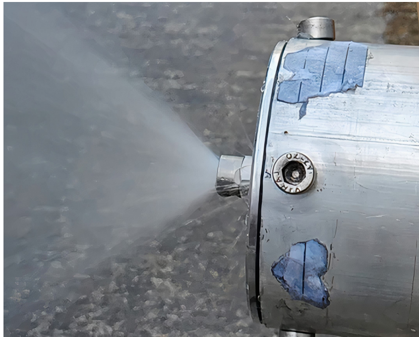
Figure 66 Hollow cone nozzle spray pattern, Source: Own
