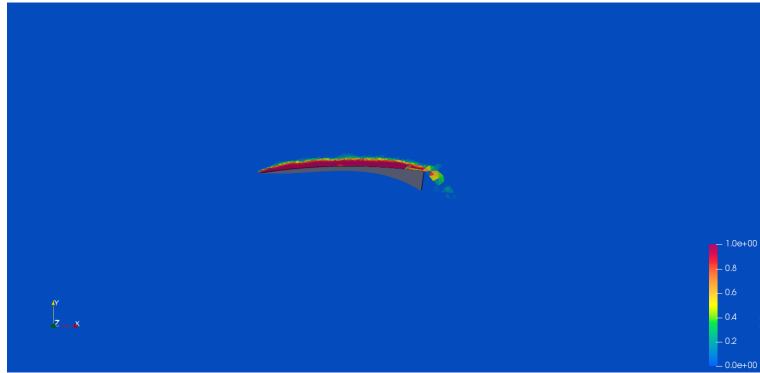
Figure 3.26: \alpha_{vap} for U = 10 \text{ m/s} .
