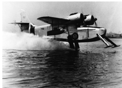
Figure 2.1: JRF5 waterski config. Figure 2.2: JRF5 hydrofoil config.
