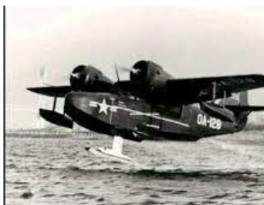
Figure 2.1: JRF5 waterski config. Figure 2.2: JRF5 hydrofoil config.
