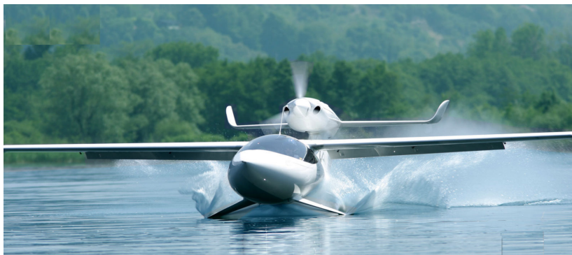
Figure 1.1: Lisa's light sports plane with its hydrofoil devices.
