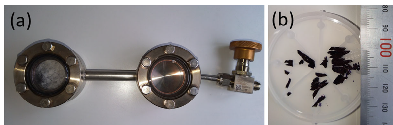
Figure 10. (a) Scaling up of the growth apparatus. (b) Obtained pentacene crystals.
