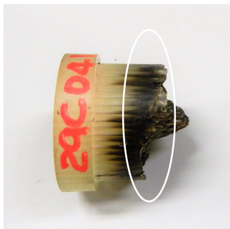
Fig. 31. The side of the fuel after the visualization experiment ( Test 11 )
