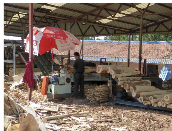
Fig. 1 Rotary lathe mill for the poplar veneer in Lianyungang, China (September 2019)
