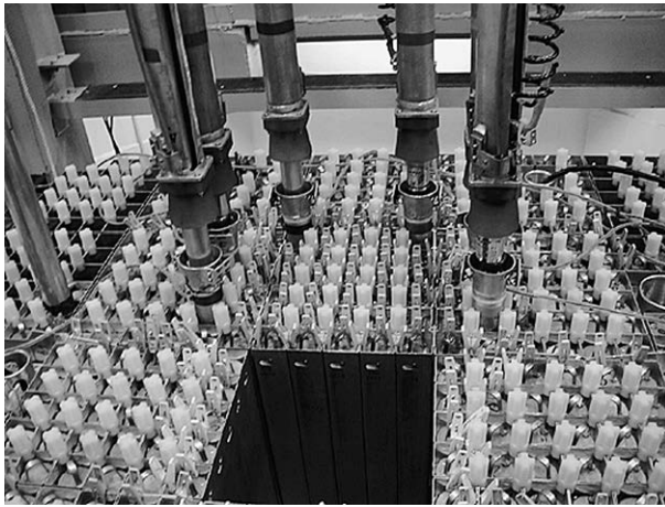
Fig. 3 Solid-moderated and -reflected core
