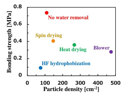
**Figure 9.** Surface particle density prior to the bonding and mechanical interfacial bonding strength for each drying process condition for the four alternative methods described in the text, along with the case with the conventional blow drying scheme.
