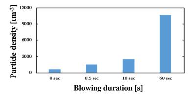
**Figure 5.** Relationship between the surface particle density and time of blowing onto the wafer surface at the blower air pressure of 0.15 MPa.
