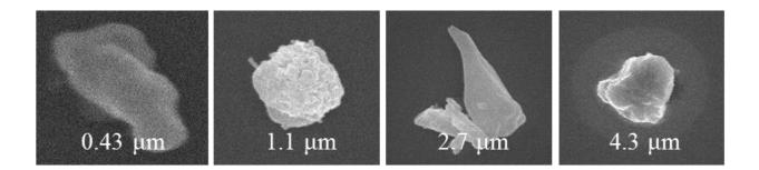
Figure 1. SEM images of typical particles adsorbed on the wafer surface from the atmosphere and their Feret diameters.
