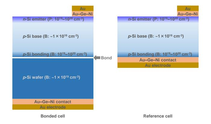
**Figure 19.** Schematic cross-sectional structural diagrams of the bonded and reference unbonded Si solar cells.
