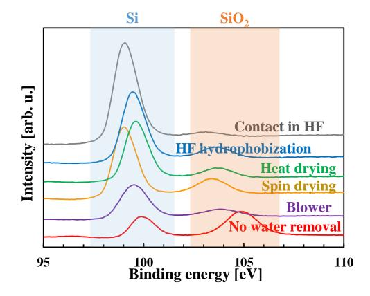
**Figure 15.** XPS spectra of the debonded Si surfaces immediately after the intentional debonding of the bonded samples obtained by the different pretreatments.
