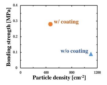
**Figure 8.** Surface particle densities and bonding strengths for the cases with and without the surface coating treatment in the cutting process.
