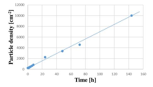
Figure 4. Typical time evolution of the areal particle density on the Si wafer surface.
