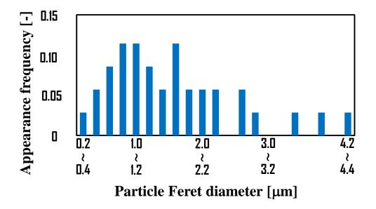
**Figure 3.** Typical distribution of Feret diameters of the particles on the Si wafer surface counted using SEM and optical microscopy for the smaller and larger regions, respectively.
