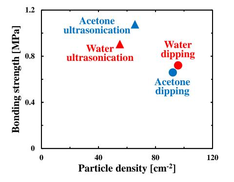
**Figure 11.** Surface particle density after each surface cleaning treatment with deionized water or acetone with and without sonication for 10 min prior to the bonding and corresponding bonding strength.
