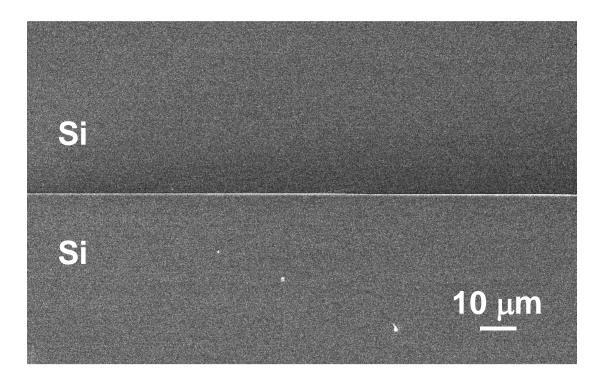
Figure 13. Cross-sectional SEM image of the bonded Si/Si interface.
