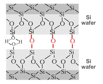
**Figure 10.** Conceptual schematic of a cross-sectional molecular view of the hydrophilically bonded Si/Si interface.
