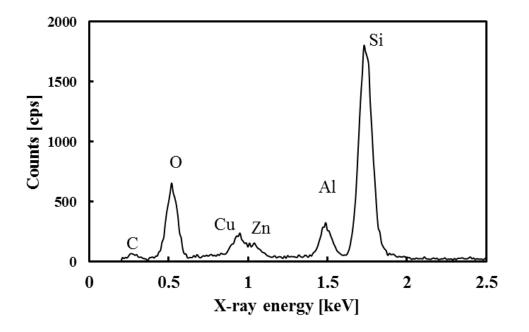
Figure 2. EDX spectrum of typical particles adsorbed on the wafer surface from the atmosphere.
