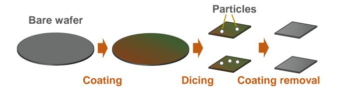
Figure 7. Flow diagram of the surface-coating scheme for the wafer-cutting process.
