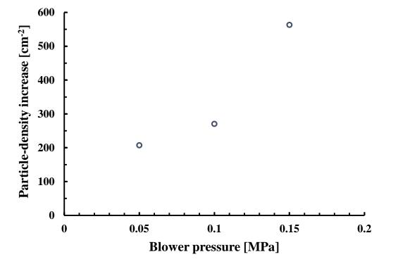
**Figure 6.** Dependence of the surface-particle-density increase on the air pressure of the blower gun for the blowing times required to complete the removal of water droplets from the Si surfaces.
