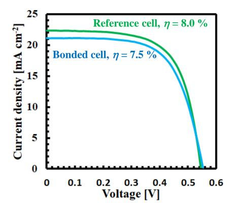
**Figure 20.** Light current–voltage characteristics of the highest-efficiency bonded and reference unbonded Si solar cells under the AM1.5 G, 1-sun illumination.
