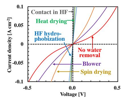
**Figure 14.** Current–voltage characteristics across the bonded Si/Si interfaces obtained by various surface treatments.
