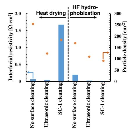
**Figure 17.** Surface particle densities (dots) and interfacial electrical resistivities (bars) for the cases with the SC-1 cleaning ( $NH_3:H_2O_2:H_2O = 13:17:70$  wt:wt:wt) for 10 min, ultrasonic cleaning in deionized water for 2 min, and without these treatments, for the preparation procedures with the heat drying and HF hydrophobization.
