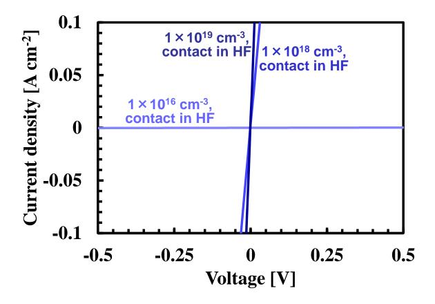
**Figure 18.** Current–voltage characteristics for the different doping concentrations in the Si wafers for the samples obtained by the procedure including the SC-1 cleaning followed by prebonding contacting in HF aq.
