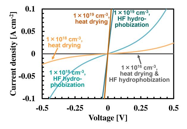
**Figure 16.** Current–voltage characteristics for the different doping concentrations in the Si wafers for the samples obtained by HF hydrophobization and heat drying.
