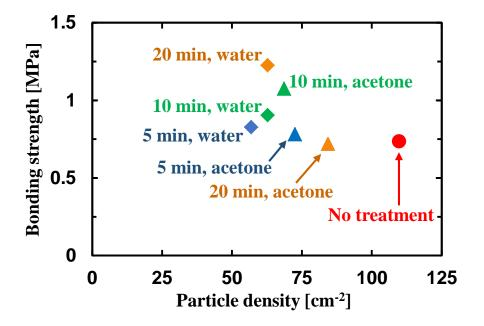
Figure 12. Surface particle density after each sonication prior to the bonding and obtained bonding strength.
