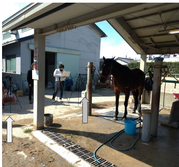
Fig. 1. Photograph of the experimental environment. The gray arrows indicate the radar device. The dotted arrow indicates the thermal imaging camera.
