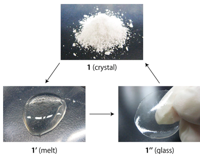
Figure 5. Photographs of [\text{Zn}(\text{HPO}_4)(\text{H}_2\text{PO}_4)](\text{H}_2\text{Im})_2 in various states. Reprinted with permission from ref 26. Copyright 2015 American Chemical Society.
