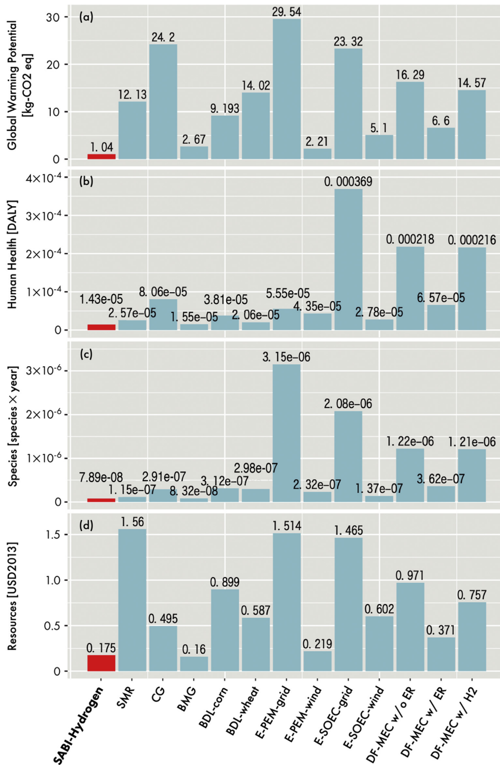
Fig. 12 – Comparison of environmental footprints: (a) Global warming potential, (b) human health, (c) species, and (d) resources.
