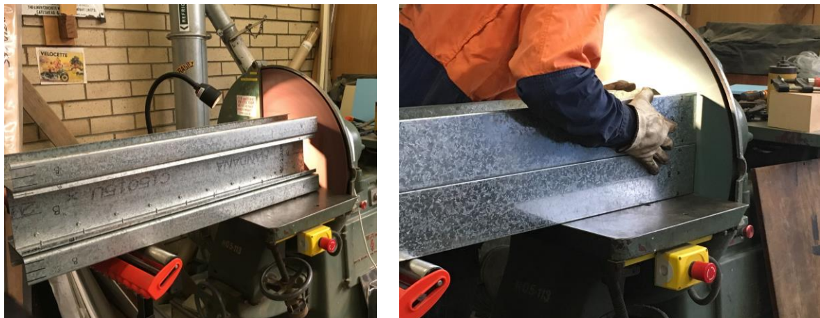
Figure 4-9: Flattening the end of specimens using a linisher
