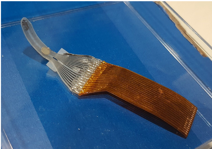
Figure 5-5 Whole array with custom made, copper-polyimide ribbon cable for connection to the stimulation/recording electronics.
