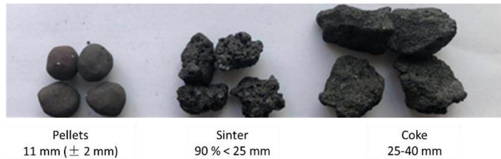
Figure 7. Blast furnace materials and the size of them: pellets, sinter and coke.
