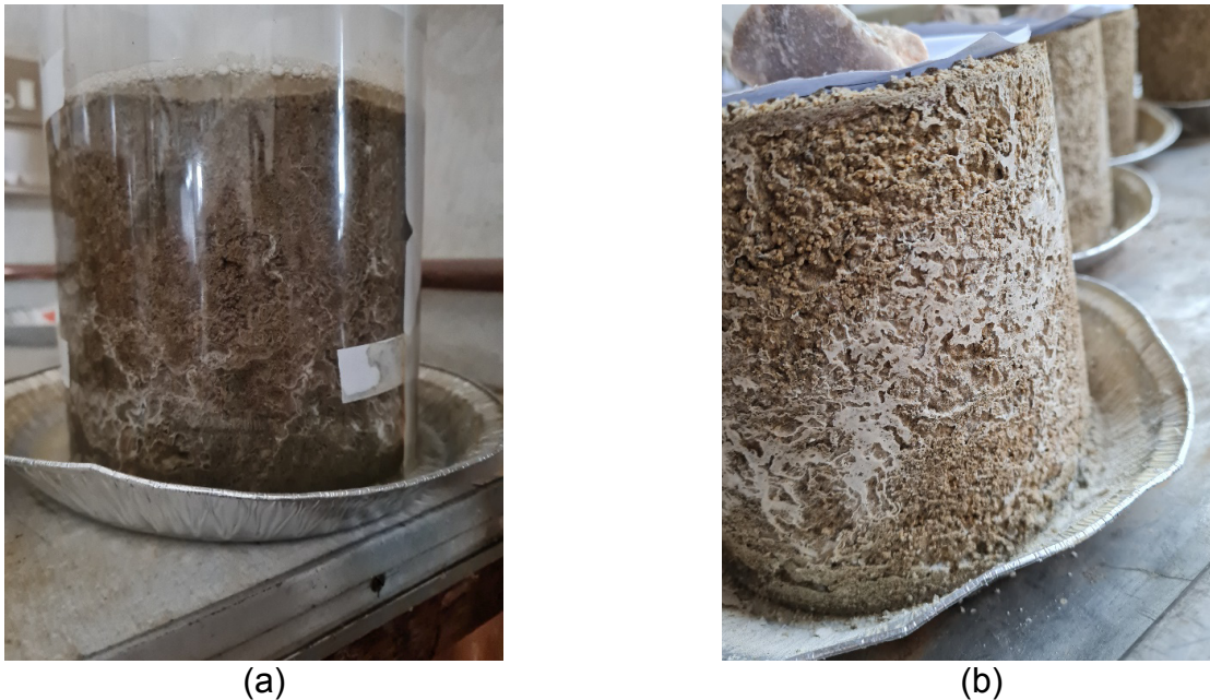
Figure 4: In situ cultivated C UCS samples (a) after two applications of cementation solution (b) after 20 days and curing
