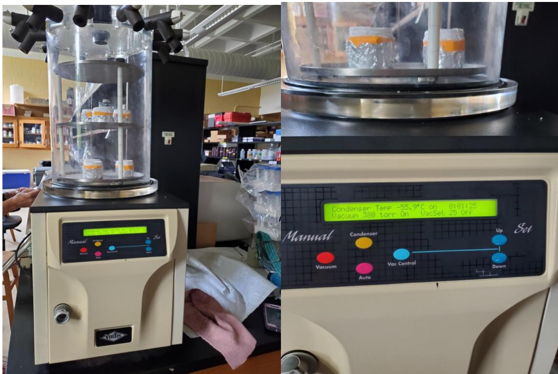
Figure D1 Freeze drying sediments; apparatus and set-up
