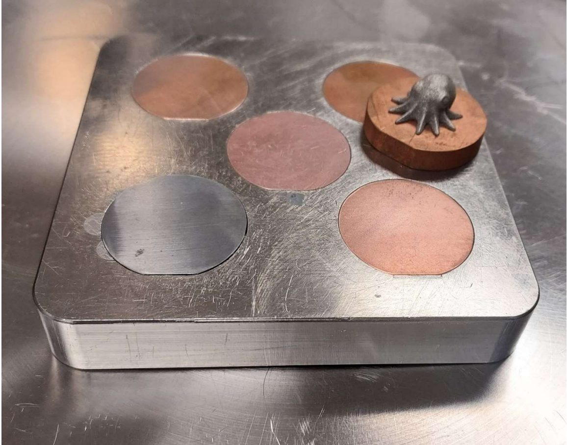
Figure 4: Build plate modified for removable pucks, with copper and molybdenum pucks loaded
