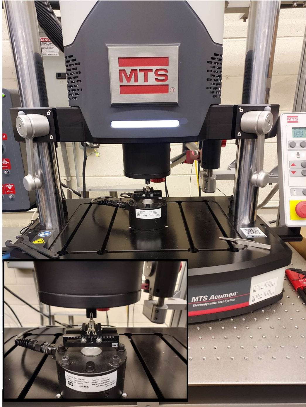
Figure 8: MTS Acumen load frame; MTS micro three-point bend fixture
