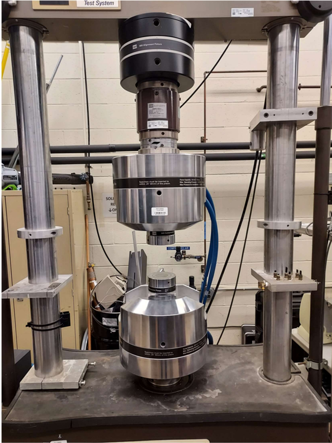
Figure 9: MTS 110-kip load frame for compression
