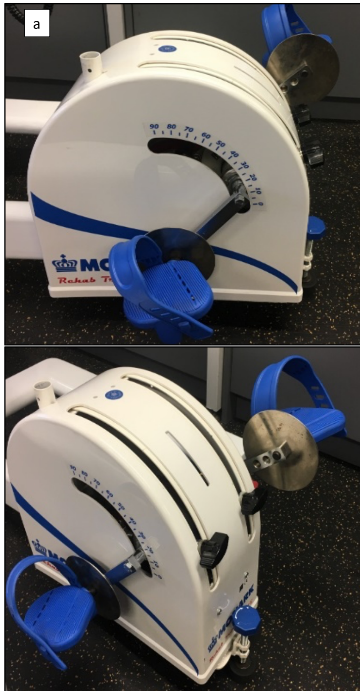
Fig 2.1a: Eccentric cycle ergometer. Retro-fitted Monarch Rehab Trainer modified by the internal inclusion of a 125 W asynchronous motor and SRM power meter in line with the externally visible pedals.
