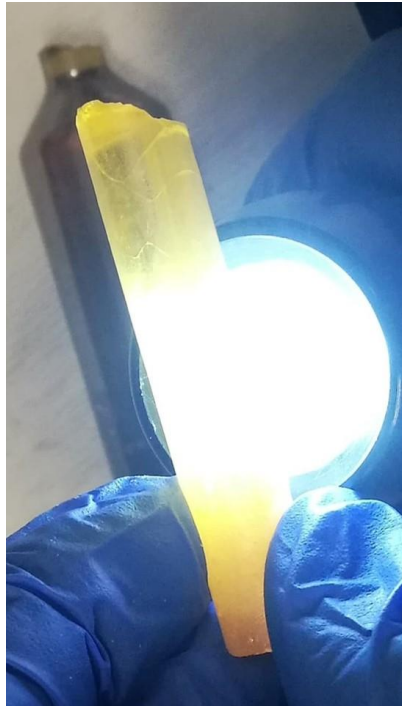
Figure 5.20 Tapered as-grown boule of Sm-PMN-PT.
