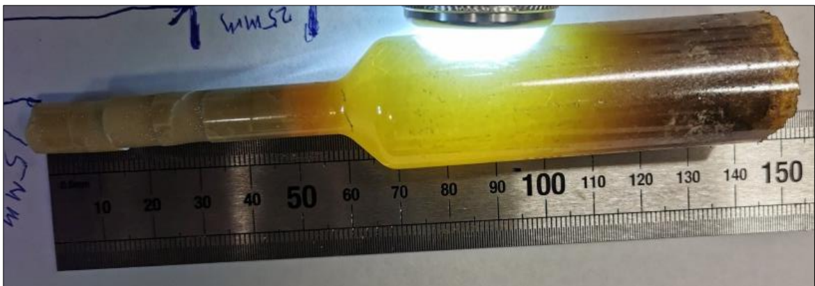
Figure 5.10 As-grown boule of PMN-PT.
