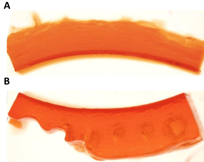
Figure 19. F-gelNB 10% 2% dye prints. Back view of positive features (A) and back view of negative features (B). Condition: f-gelNB 10% 2% dye 65 mJ/cm 2 . Pictures were taken at the microscope with 1.5x magnification.
