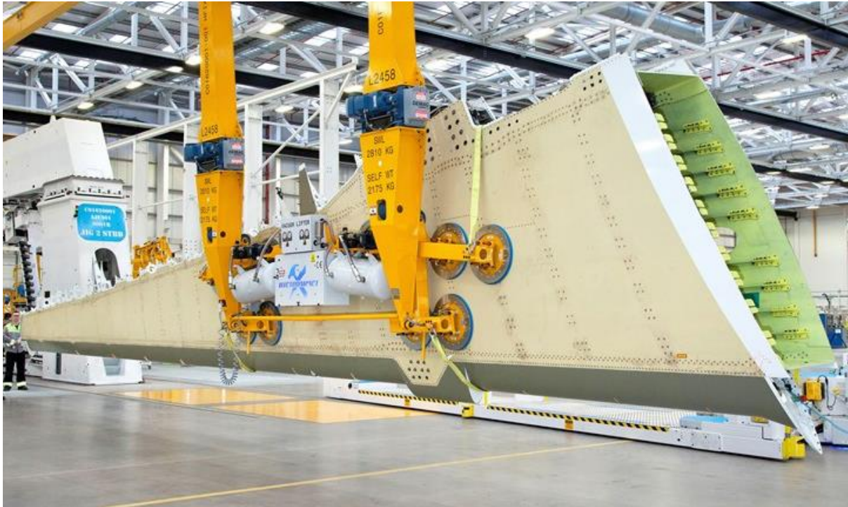
Figure 1.1: Airbus A220 wing at the Bombardier Belfast facility with bottom cover and ribs shown, the wings for the Airbus A220 are manufactured using liquid resin infusion in combination with continuous carbon fibre reinforcement
