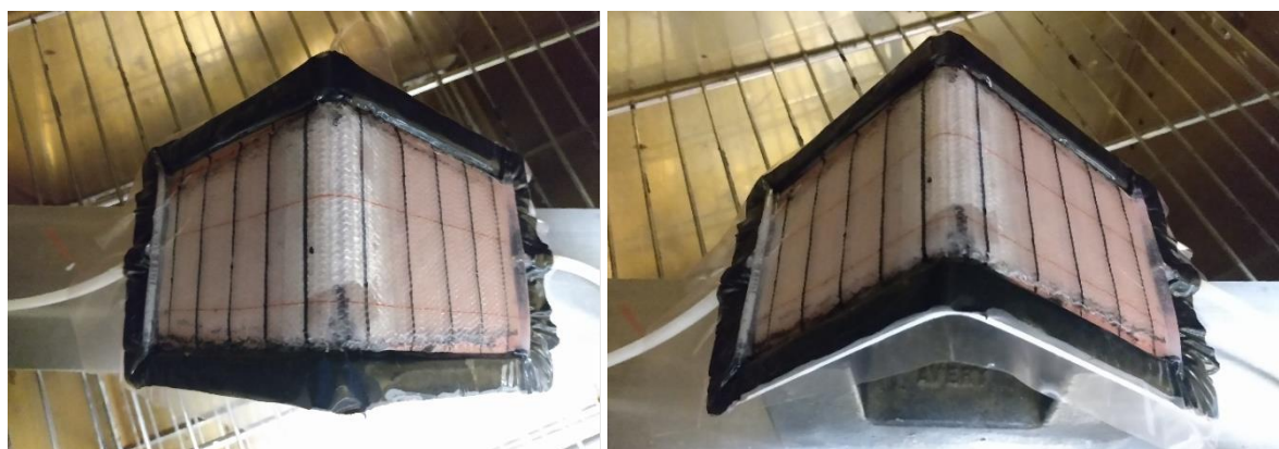
Figure 7.15: Test sample showing leakage into isolated zone, there is only partial intrusion of resin which is visible are the bottom edge of the corner, the remainder of the corner region remains dry. Sample shown after curing.
