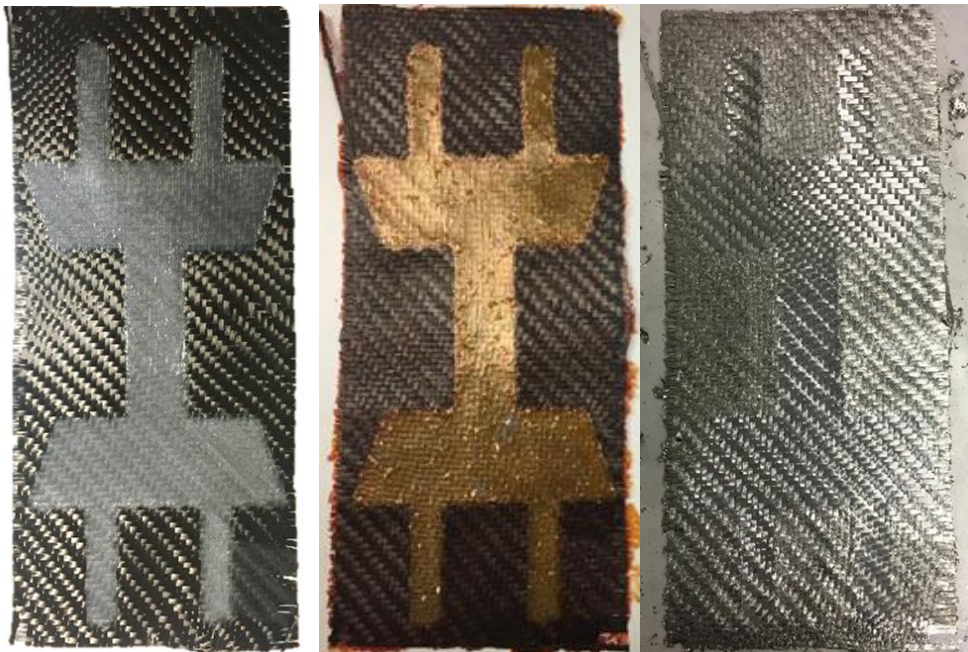
Figure 1.4: The various stages of the carbon aerogel pyrolysis process utilizing carbon aerogel, left: the shape of the formable zone is masked with resin film (these are the areas where the yarns are no longer visible); centre: the sample is infused with carbon aerogel precursor; right: the sample after pyrolysis now ready for forming and further infusion of structural resin
