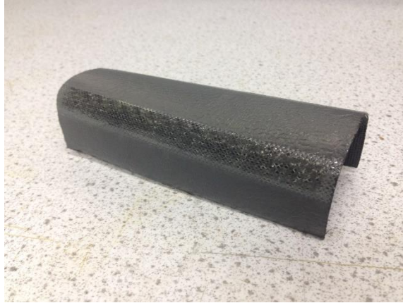
Figure 7.12: Multi-matrix trial demonstrator, this is only a proof of concept and therefore is not infused with carbon aerogel, however the partitioning between distinct formable and flat zones can be seen
