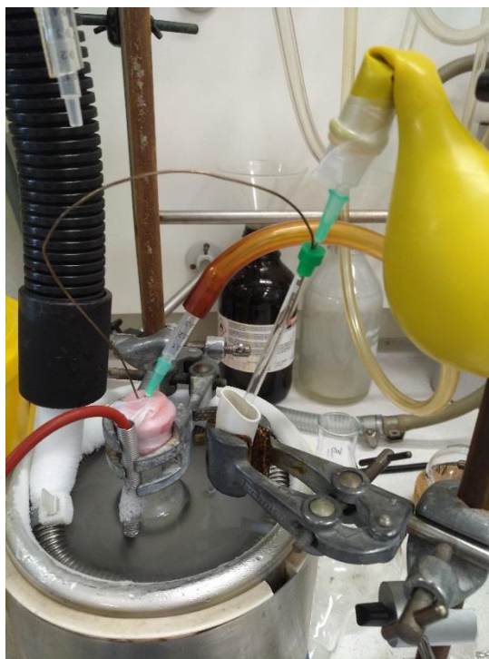
Figure 8. Reaction set-up and subsequent transfer of the reaction mixture into an NMR tube via a cannula at -78\text{ }^{\circ}\text{C} .
