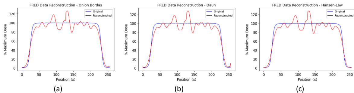
Figure 4.18. D_{max} profile comparison for FRED integrated projection data. The Onion Bordas (a), Daun (b) and Hansen-Law (c) methods of inverse Abel transform were used for the reconstruction of a 40mm TOPAS simulated proton beam distribution, with a Gaussian filter ( \sigma = 5 ) used to smooth to the projections before reconstruction.
