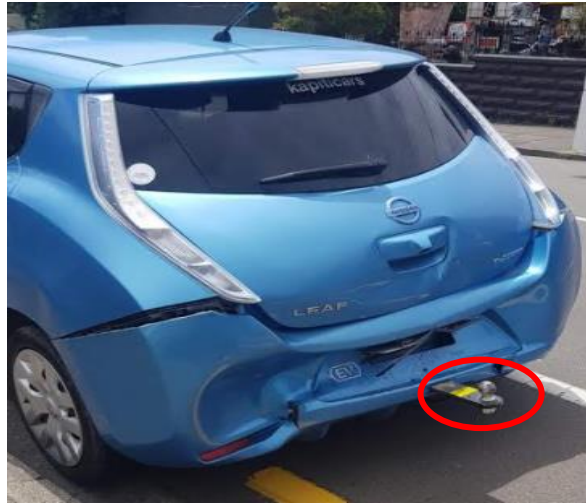
Figure 26 - Damaged caused in Nissan Leaf due to towing
