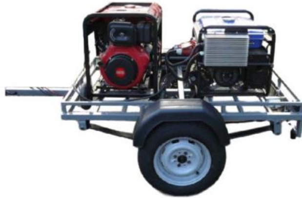
Figure 4 - Range Extender Trailer with motor and generator (Lebkowski, 2019)
