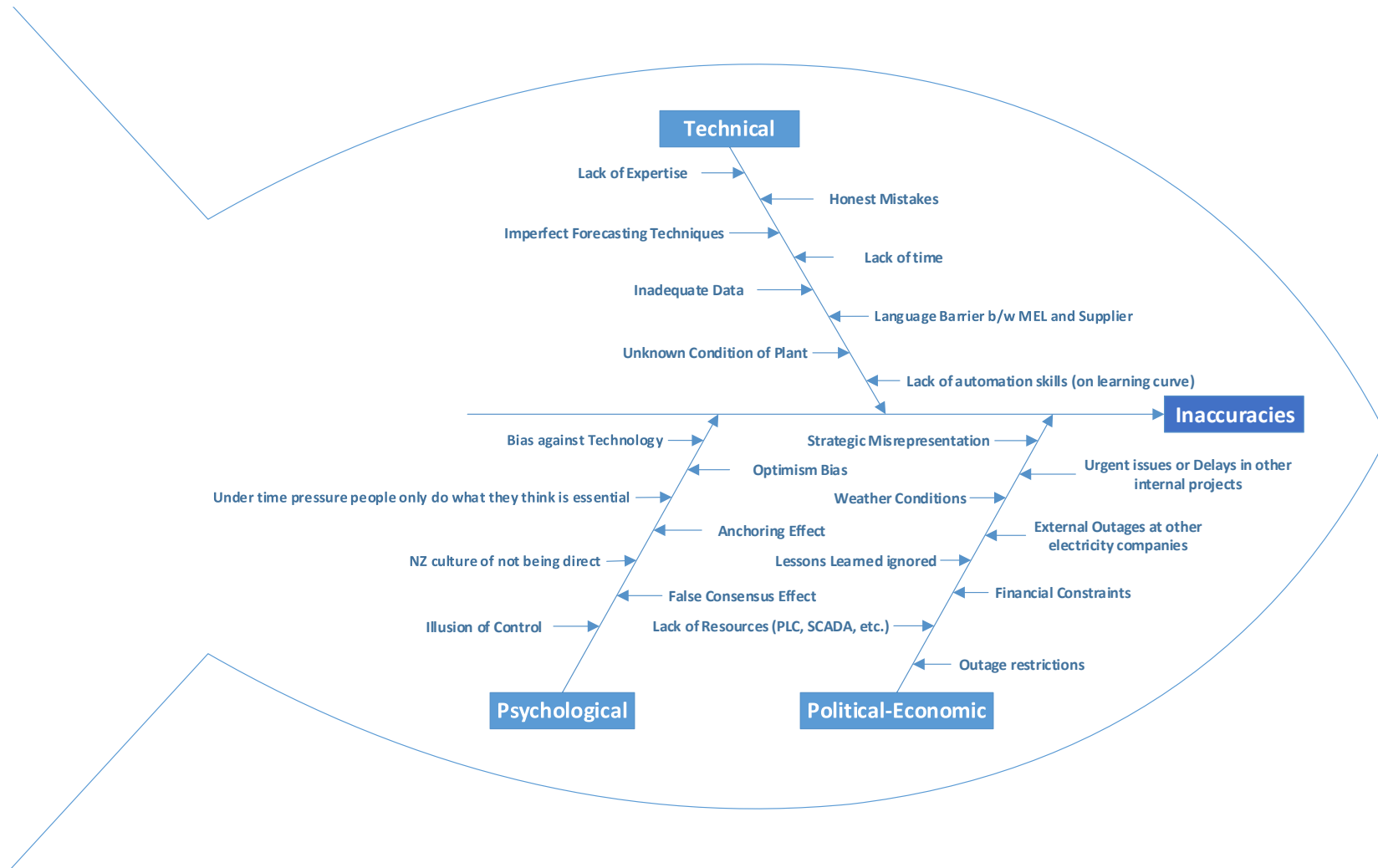
FIGURE 10: ISHIKAWA DIAGRAM OF ROOT CAUSES FOR INACCURACIES IN THE PROJECT DELIVERY OF CASE STUDIES
