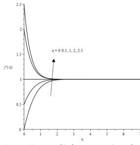
**Fig. 6.** Velocity profile for various values of  $\mathcal{E}$  when Pr = 21, M=0.5,  $\lambda = 0.1$
