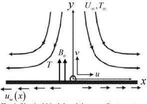
Fig. 1. Physical Model and the coordinate system
