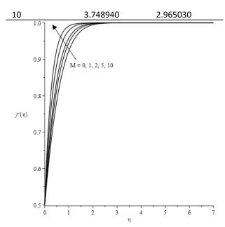
**Fig. 4.** Velocity profiles for various values of *M* when Pr = 21,  $\lambda = 1$ ,  $\varepsilon = 0.5$
