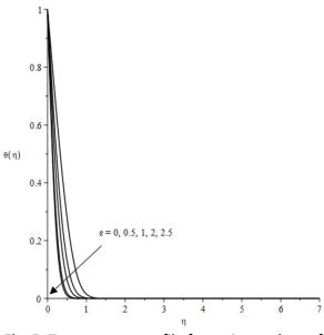
Fig. 5. Temperature profile for various values of  ${\cal E}$  when Pr = 21, M=0.5,  ${\cal A} = 0.1$
