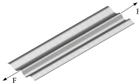
Figure 4. Wrinkling of initially planar UD ply due to shear buckling in off-axis tensile test.
