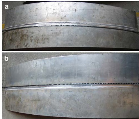
Fig. 5 The result of the product: (a) without control; (b) with automatic control
