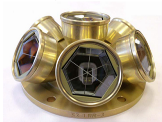
Laser retroreflector on Sentinel-3
