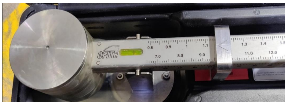
Figure 7. 4 - Measurement of mud density before and during wear tests
