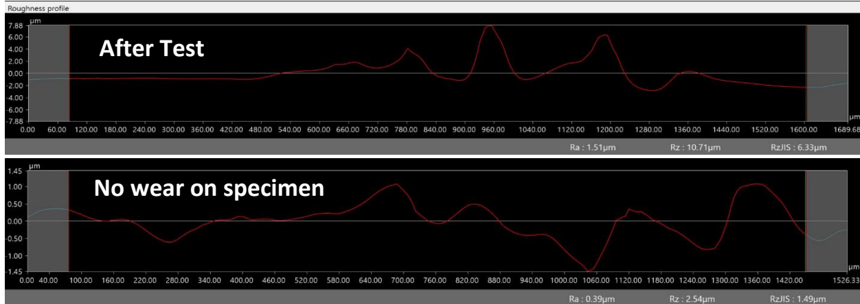
Figure 8. 9 - Roughness profile for steel casing (with water) pre-test vs after test
