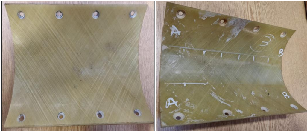
Figure 7. 14 - Glass fiber casing specimen before (left) and after (right) Test No. 10
