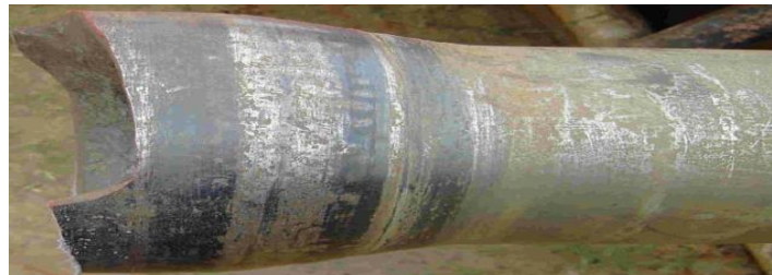
Figure 2. 9 - Shiny polished layer on a failed tool joint pin section [16]
