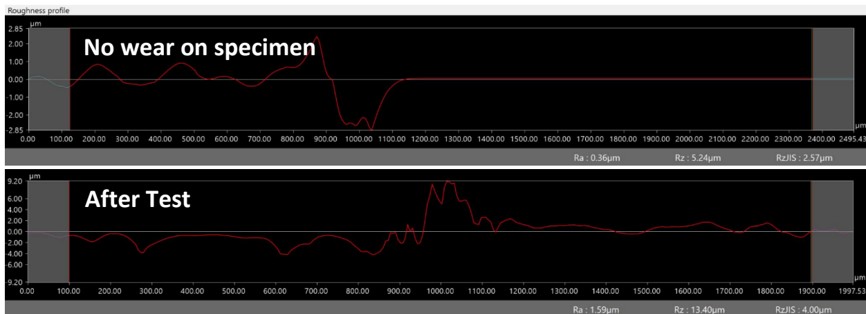
Figure 8. 10 - Roughness profile for steel casing (with mud) pre-test vs after test
