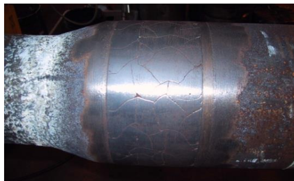
Figure 3. 20 - TJ Hardbanding Arnco 350XT® with a smooth hard-face [38]
