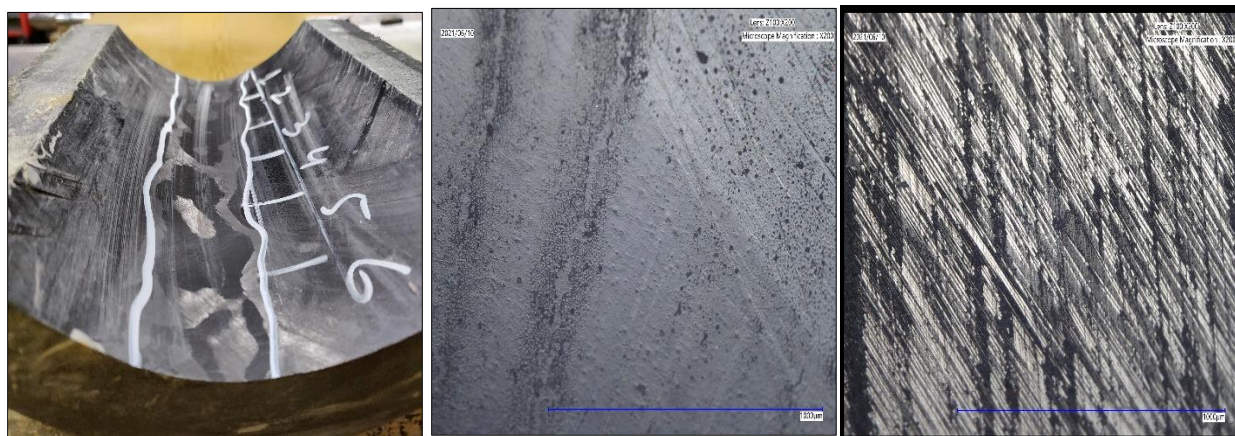
Figure 7. 21 - Worn specimen after 480 min (left) and its micro image at 200X before test (middle) and after test (right)
