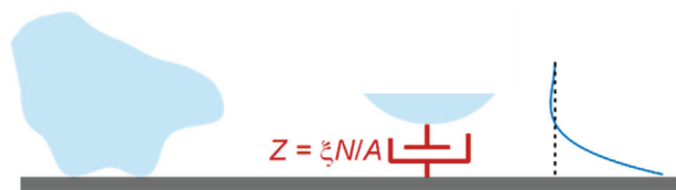
Figure 6. A shift in bandwidth, only, with \Delta\Gamma independent of overtone order (as in Figure 5H) can be attributed to a dashpot. This behavior may be caused by narrow, soft links to large clusters. The geometrical configuration is depicted on the left. The center shows the mechanical equivalent circuit. The blue line to the right sketches the decaying shear wave. \xi = F/\nu is the friction coefficient of the bridge, where F is the transverse force and \nu is the velocity of the substrate. Both F and \nu are complex amplitudes. N/A is the number density of adsorbed clusters. Z is the total load impedance generated by the ensemble of bridges.
