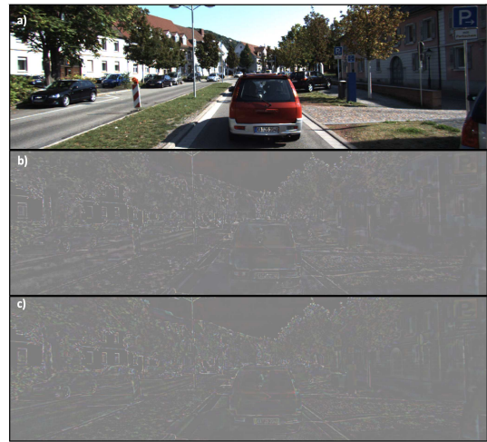
Fig. 3. a) A frame from the original KITTI MoSeg dataset, and the loss per pixels between the original frame and the compressed frames ( QP=51 ) using (b) AVC and (c) HEVC standards.
