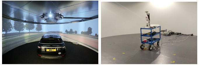
Fig. 1. Left) Image showing how the 3xD simulator operates as a simulator for driver-in-the-loop applications. Right) Image showing how the 3xD simulator at WMG was adapted to carry out interference measurements. In the image there is a single LiDAR (i.e. the victim LiDAR) mounted on a trolley in the centre of the simulator
