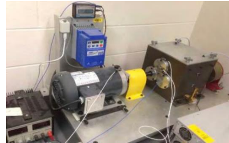
Fig. 6. Planetary gearbox fault simulation platform of case 1
