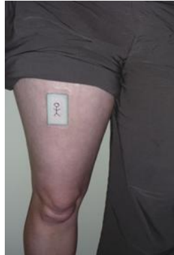
Figure 2.2 activPAL device attached to a participant's thigh (source: Edwardson et al., 2017)
