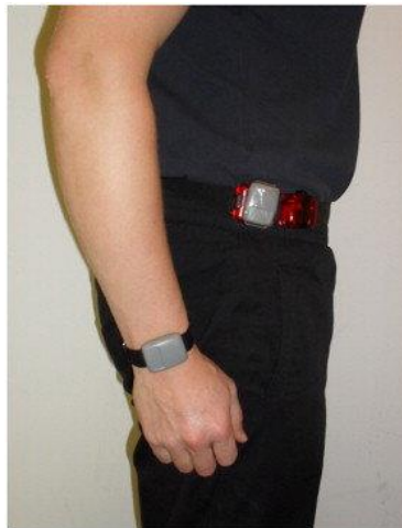
Figure 2.3 Positioning of the Actigraph GT3x (source Rowlands & Stiles, 2012)
