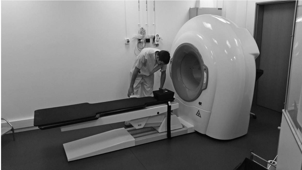
Figure 4. CT scanner (X-ray computed tomography). Copyright: C. Moulhérat.
