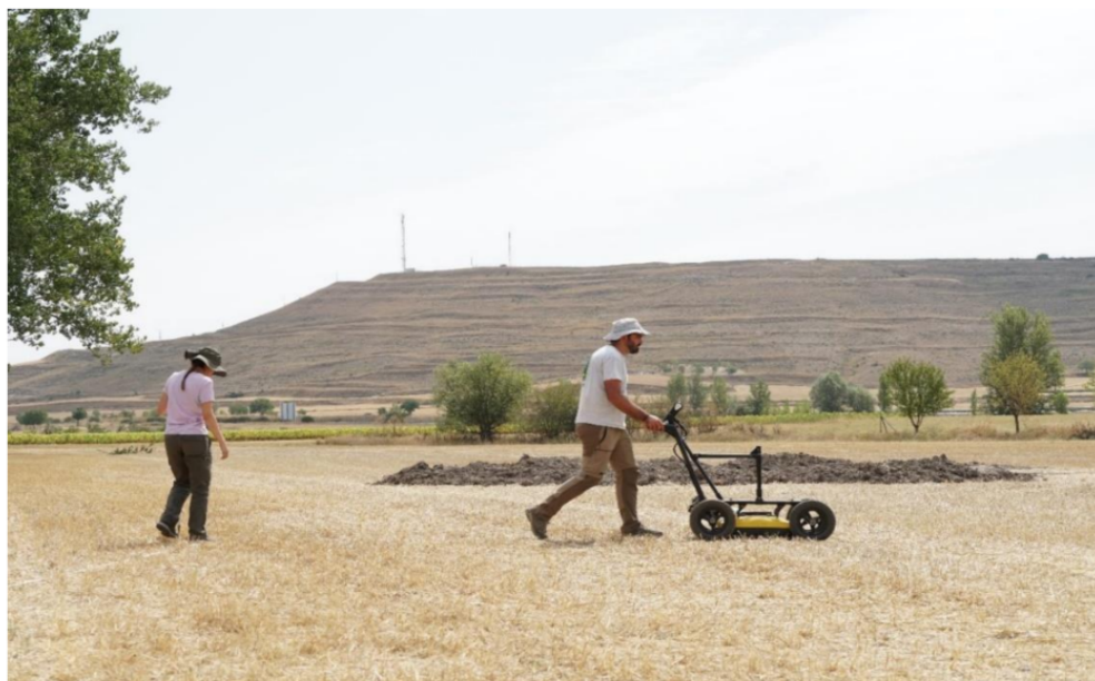
Figure 3. GPR survey in August 2021 at Villa María with Noggin 250 Mhz. In the background, the oppidum of Cerro de Castarreño, Sasamón.
