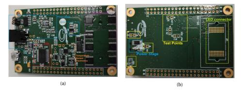
Figure 4.12: Pictures of the top and bottom sides of the implemented LED driver PCB for the LEDs used in the minimum sized LED microscope.
