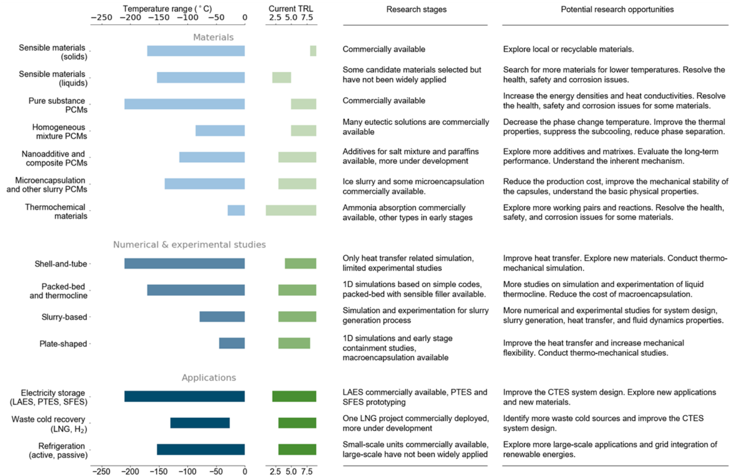
Figure 1.4: Development stages and research directions of CTES in sub-zero temperature ranges [7].
