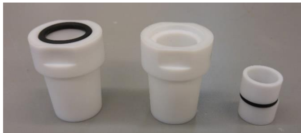
Figure 3.38. Teflon adaptors to use Schlenk tubes in the photoreactor.
