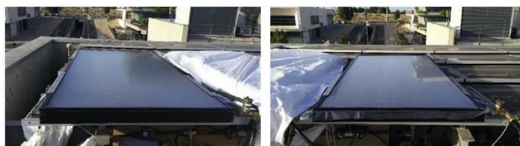
Fig. 6. a) solar collector b) modified solar collector used as radiative cooling device.
