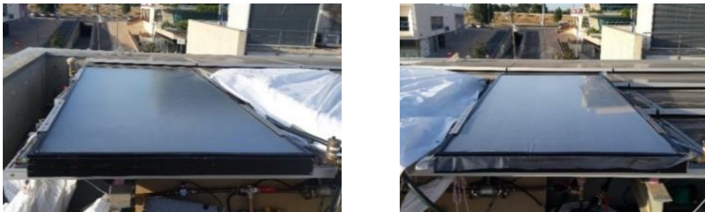
Figure 12 – Solar thermal collector plate (left); radiative cooling plate (right)
